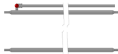
SUPPORT FRAME Ø 42 mm (2 tubes Ø 42 mm, 1 control linkage Ø 27 mm, 1 handle Ø 27 mm, 4 calf ends)
