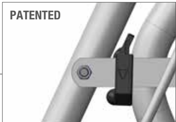
RAZ SYSTEM: RETURN TO ZERO OF MOVING ARMS MAKING THEM SILENT IN THE OPEN POSITION
